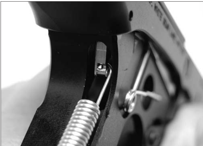
Figure 30. Incorrect mainspring attachment
