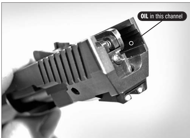
Figure 20. Ejector Cam oiling point
