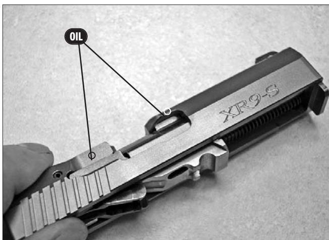
Figure 19. Extractor/Locking Lug oiling points
