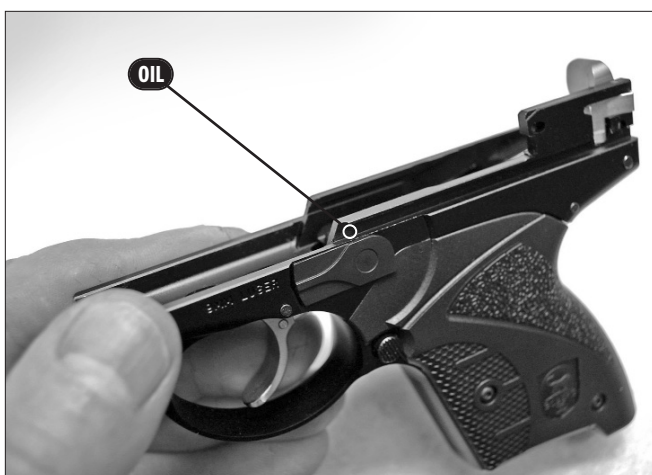
Figure 15. Left Slide Rail oiling point
