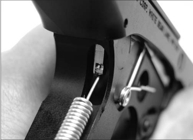
Figure 29. Correct Mainspring attachment
